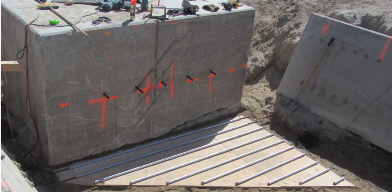
Figure 3-10: Roller foundation for 15° and 30° wedges (Marsh, 2013)
