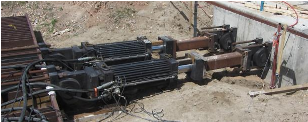
Figure 3.9: MTS hydraulic actuators
