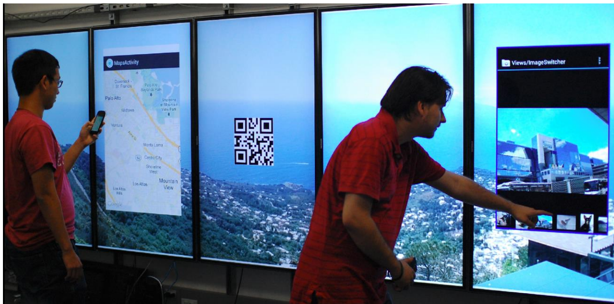
Figure 8 – The Open Project framework allows slightly modified applications to share themselves to a shared display from an Android device.
