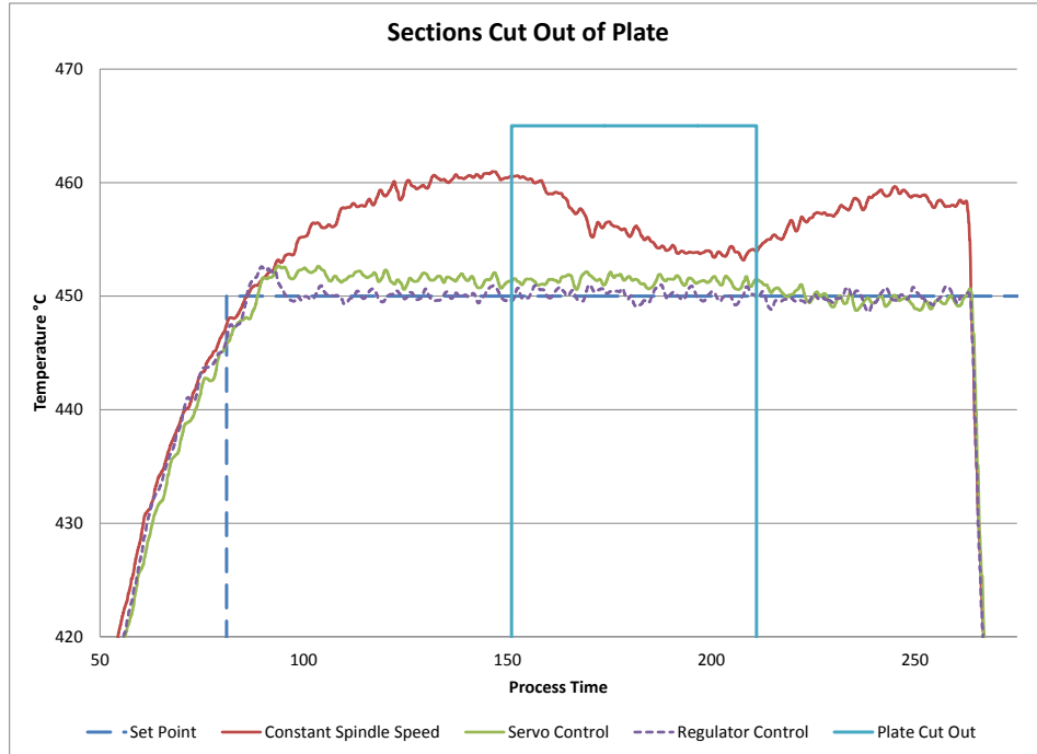
Figure 2.17: Side sections of a plate were removed to simulate a geometric disturbance.
