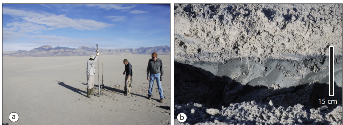
Figure 2.- Location 1. A) Field assistant using the hand-driven percussion auger at Rozel Point, Great Salt Lake. B) Excavation pit dug at Rozel Point displaying thickness of ooids and sharp contact between ooids and lake muds.
