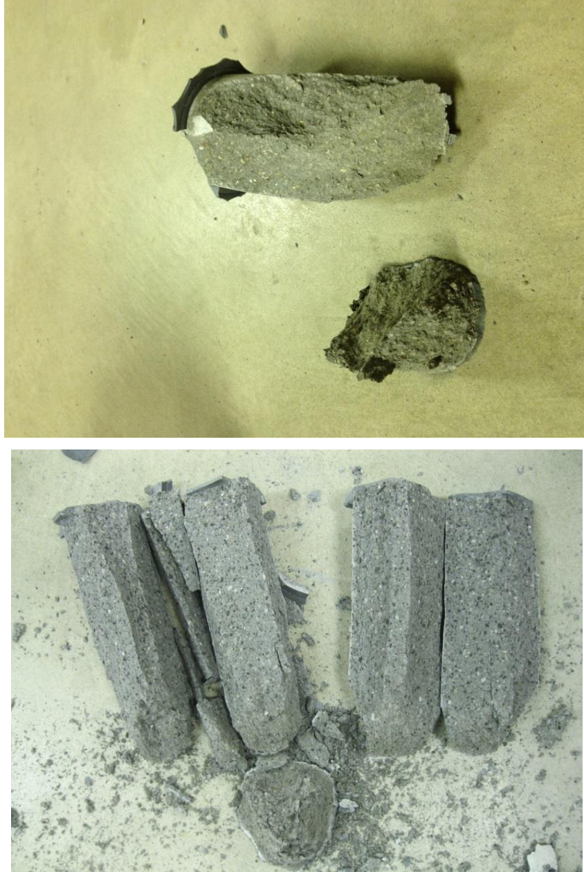
Figure 21. Normal-Weight Fine Grout Failure and Light-Weight Fine Grout Failure
