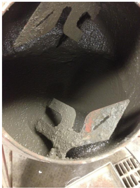
Figure 5. Concrete Mechanical Mixer with Grout Type 3
