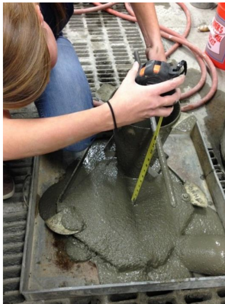
Figure 7. Grout Slump Measurement with Grout Type 3
