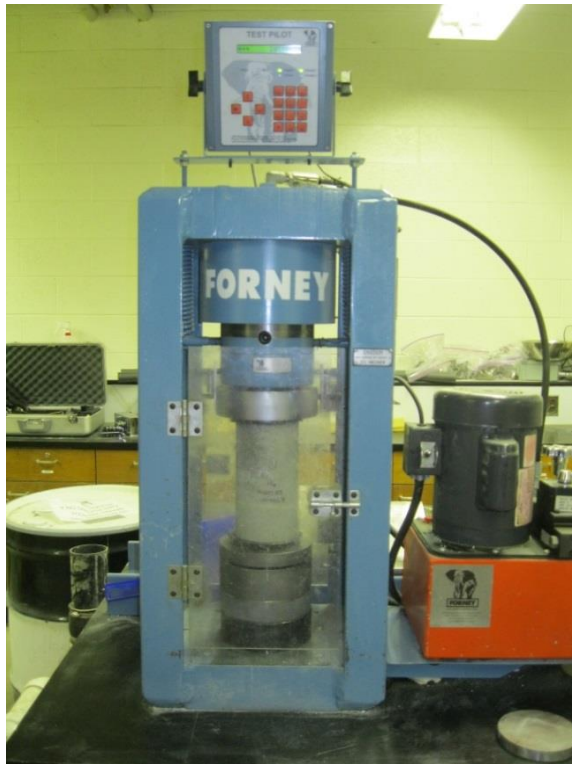
Figure 13. Grout Specimen Compressive Testing
