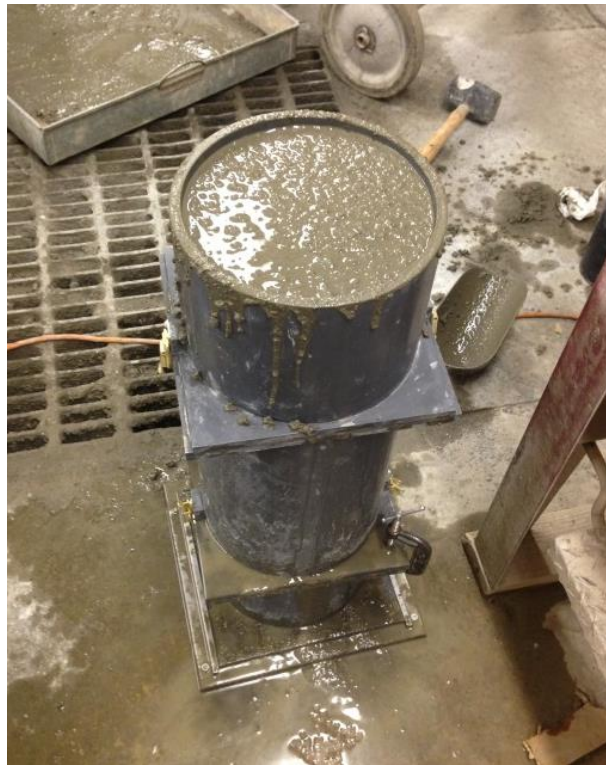
Figure 10. Segregation Column with Grout Type 5
