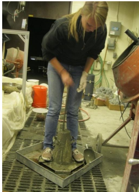
Figure 6. Slump Cone with Grout Type 6
