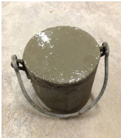
Figure 8. Unit Weight Bucket with Grout.
