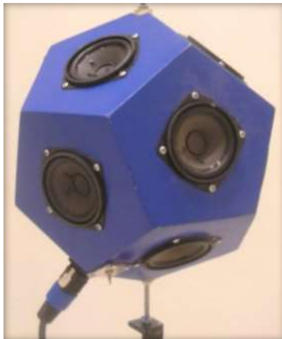
Figure 3.1 The dodecahedron loudspeaker used in the investigation. It is composed of 3-inch drivers mounted on 12 regular pentagonal faces. Ideally, all drivers radiate in phase and with equal amplitude.
