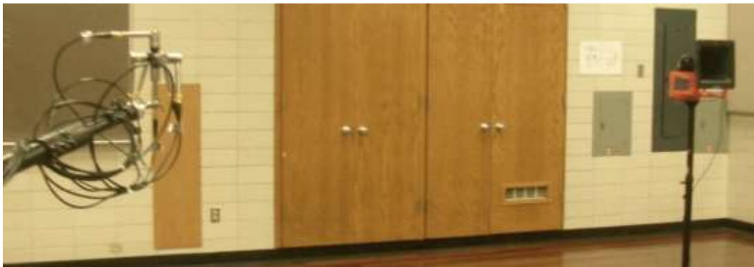
Figure 4.2 Example configuration for step 6. The horn-loaded compression driver is the source under test. The energy density probe is located at position 1 (a) and position 2 (b). Both positions are along the same arbitrary angle relative to the source under test.
