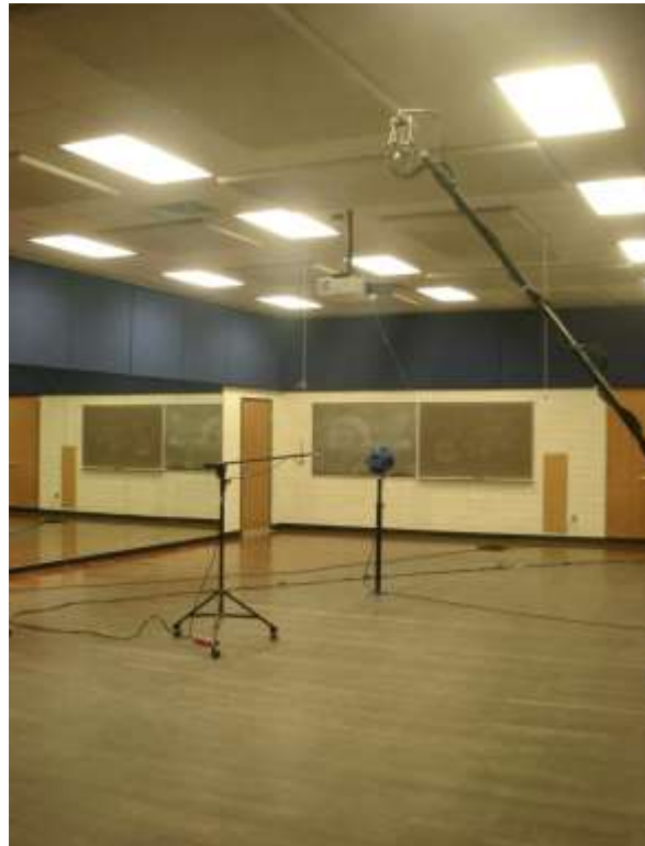
Figure 3.13 Experimental configurations for testing the GSPF in semi-reverberant spaces. The probes were moved after each source-receiver measurement and repeated until six spatial energy density measurements were taken with each probe. (a) Classroom (small room). (b) Dance studio (large room).
