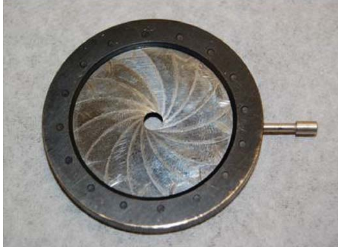
Figure 4.3: Photograph of a circular diaphragm aperture used to release ball bearings and ice balls consistently.
