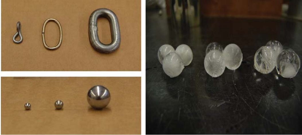
Figure 5.1: Photographs of steel chain links, steel ball bearings, and ice balls of three different sizes used as impactors.
