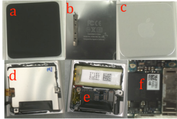
Figure 5.1 Images of an Apple iPod nano. (a) touchscreen, (b) back cover, (c) clip, (d) metal sheet, (e) circuit, and (f) circuit
