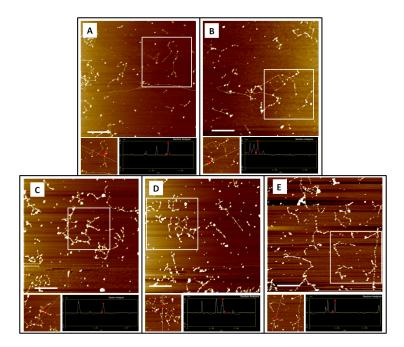
**Figure 2.2** Influence of Pd activation time on surface DNA after seeding. Activation times are (A) 2, (B) 5, (C) 10, (D) 30 and (E) 180 min. DMAB reduction for 1 min was done after activation. Height scale: 6 nm. Scale bars: 1 μm. (Left insets) Views of the white squares marked in each image, with the white lines showing the paths of the cross-section traces. (Right insets) Cross-sectional traces along the indicated paths.
