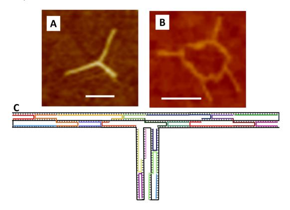
**Figure 1.4.** DNA origami method for fabricating nanostructures. (A-B) AFM images of "T"-shape and circular circuit DNA origami. Scale bar for both images: 100 nm. (C) Schematic of DNA origami layout to fold a "T" shape using the caDNAno program. The ssDNA scaffold that goes across the area of the shape is immobilized by staple strands.
