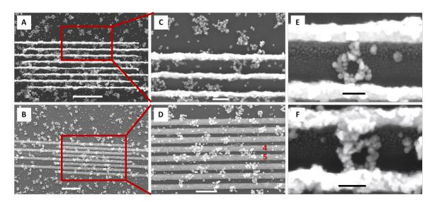
**Figure 3.8** SEM images of Au metallized CC structures after depositing Au electrodes for electrical conductivity measurements. (A-B) Large area views of the surface after electrode deposition. (C-D) Zoomed-in images of selected areas in (A-B). (E-F) Highly zoomed views of Au CC structures between Au electrodes. Scale bars: (A-B):  $1 \mu m$ ; (C): 200 nm; (D): 500 nm; (E-F): 100 nm.
