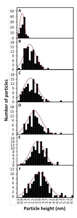
**Figure 3.2** Height distribution analysis from AFM data before and after seeding steps. Data were obtained by AFM section analysis with more than 100 measurements for each seeding condition. (A-F) Histograms and Gaussian distribution for 0-5 seeding steps. The mean heights and standard deviations are (A) 1.0
