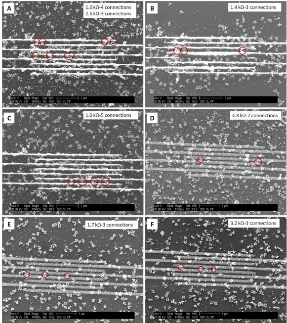
**Figure 3.10** SEM images of Au-metallized DNA origami structures between electrode pairs. (A-C) Metallized using only commercial electroless plating solution. (D-F) Metallized using two plating steps.
