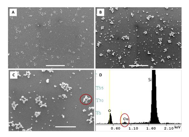
**Figure 3.7** Characterization of metallized CC DNA structures on a Si surface. (A) SEM image of a  $4 \times Pd$  seeded sample after 10 s of commercial Au plating solution treatment. (B-C) SEM images of structures plated with copper for 1 min after the Au plating pre-treatment in (A). (D) EDX of the circled structure in (C). Scale bars: (A-B): 1  $\mu$ m; (C): 500 nm.
