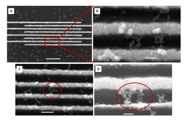
**Figure 3.11** SEM images of Cu metallized DNA origami CC structures interfaced with Au electrodes for electrical conductivity measurements. (B) Zoomed-in view of (A). (C) Zoomed image of a single Cu metallized CC structure (circled in red) between electrodes. (D) A highly zoomed image of a Cu-CC structure circled in red. Scale bars: (A) 1 μm; (B, D) 100 nm; (C) 200 nm.
