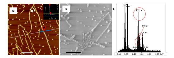
**Figure 2.5** DNA-templated Pd nanowires formed through Pd activation and seeding, followed by Pd plating for 10 min. (A) AFM image of continuous Pd nanowires on mica; inset: height analysis along the blue line in (A). Height scale: 80 nm. (B) SEM image of Pd nanowires on mica. (C) EDX spectrum of nanowires in (B) by spot scanning. Scale bars for (A–B): 1 μm.
