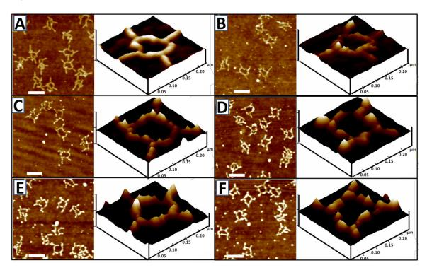
**Figure 3.1** AFM height and 3D images of DNA origami CC structures on Si. (A) Unseeded structures. (B) 1, (C) 2, (D) 3, (E) 4, and (F) 5 palladium seedings. (Left) Height images; height scales: 6 nm; scale bars: 200 nm. (Right): 3D-view AFM images of individual structures. Height scale: 6 nm.
