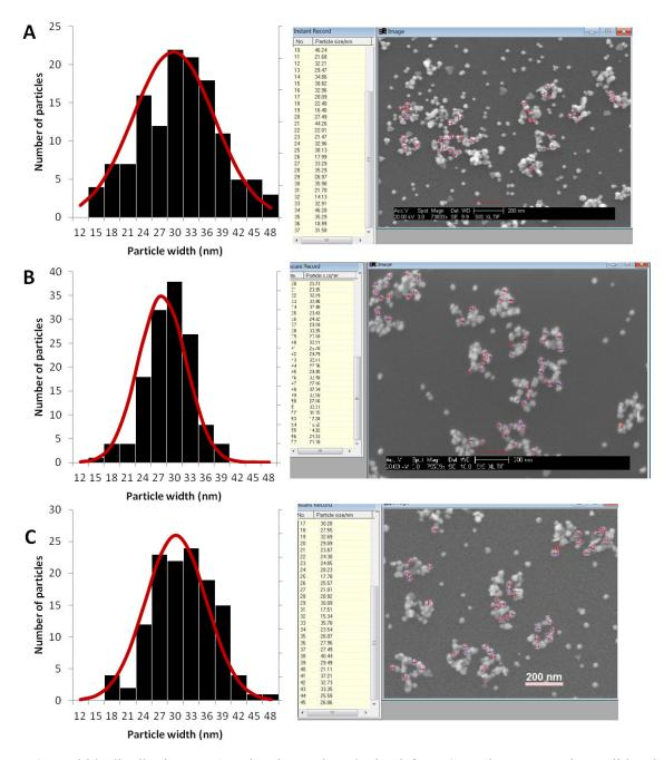
**Figure 3.5** Width distribution on Au plated samples obtained from SEM images. Each condition had more than 100 measurements from different samples. 10 min commercial Au electroless plating on (A) 3, (B) 4 and (C)  $5 \times Pd$  seeded samples. Mean particle widths and standard deviations were  $29.6 \pm 7.7$ nm,  $27.6 \pm 4.6$  nm, and  $30.0 \pm 5.7$  nm.
