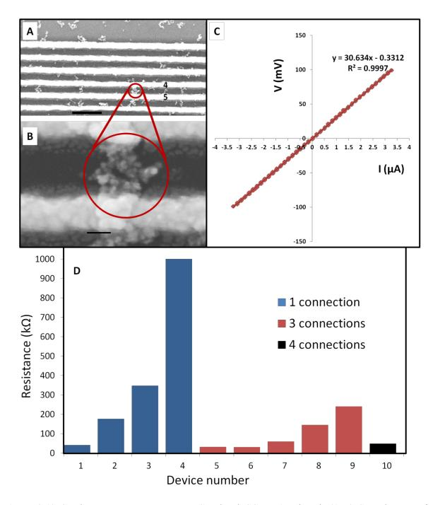
**Figure 3.12** Conductance measurements on Cu plated CC DNA origami. (A-B) SEM images of Cu nanostructures between electrodes. Scale bars: (A) 500 nm; (B) 50 nm. (C) Current-voltage plot obtained between Au electrodes 4 and 5 in (A). (D) Histograms of measured resistance values between electrode pairs having a single structure (blue), three structures (red), or four structures (black) between electrodes.
