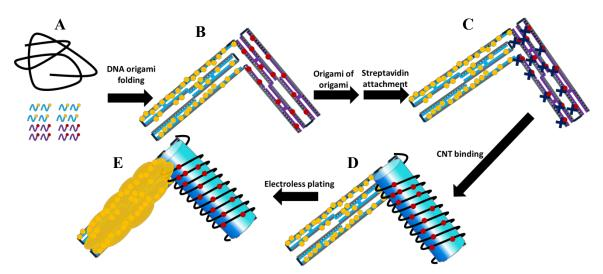
**Figure 4.3** Schematic of metallization of CNT attached super DNA origami structures. (A-B) DNA origami formation in which four different DNA origami are folded individually, with specific locations having Pd(0) or biotin. (C) Further super DNA origami folding and then attachment of streptavidins onto biotin sites. (D) CNT binding onto DNA origami site selectively. (E) Electroless plating of the seeded part of DNA origami.
