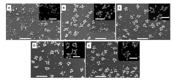
**Figure 3.4** SEM images of CC DNA origami Au plated for 10 min for (A-E) 1-5 Pd seedings. Scale bars: 500 nm. Insets are zoomed in images for each condition. Scale bars for insets: 200 nm.
