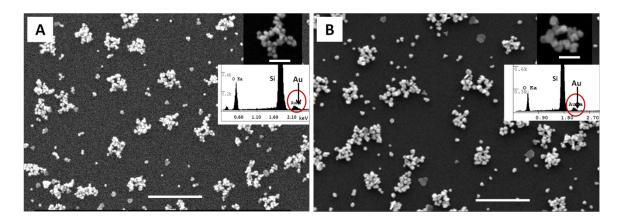
**Figure 3.6** SEM images of Pd seeded CC structures made by (A) Au plating with a commercial solution only; or (B) Au plating with a commercial solution followed by Au plating using a published approach. Insets are highly zoomed images and EDX spectra of the zoomed region. Scale bars: 500 nm. Scale bars for insets: 100 nm.
