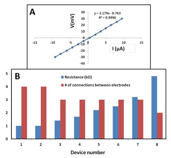
**Figure 3.9** Conductance measurements on Au-plated DNA origami CC samples. (A) A typical current-voltage plot obtained of Au plated DNA origami bridging between Au electrodes. (B) Histogram of measured resistance values for 9 electrode pairs having Au-coated structures connecting them.
