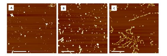
**Figure 2.4** AFM images of metallized lambda DNA after Au plating for 5 min in a bath having (A) no Mg<sup>2+</sup>, (B) 2 mM Mg<sup>2+</sup> and (C) 10 mM Mg<sup>2+</sup>. Scale bars: 1 μm. Height scale: 80 nm.
