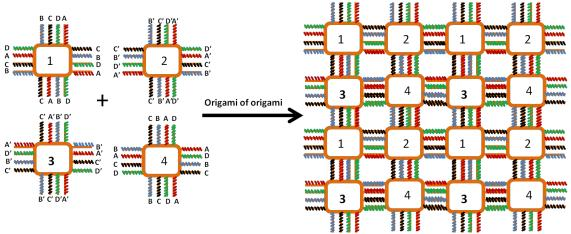
**Figure 4.1** Origami of origami to form ordered circuit structure. Bridging strands (sticky ends) with different colors indicate different sequences. A-A', B-B', C-C', and D-D' are complementary with each other.
