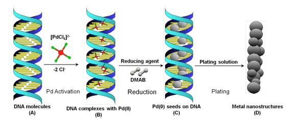
**Figure 2.1** Schematic of Pd seeding and plating on double-stranded DNA. Pd(II): red; Cl: green; Pd(0): silver. (A) Double-stranded DNA; base pairs are represented by yellow bars. (B) Interaction between DNA and Pd(II) (in the form of  $PdCl_4^{2-}$ ) to form complexes. (C) Pd seeds on DNA strands after reducing. (D) More metal is deposited to form nanostructures on the Pd(0) seeds upon treatment with plating solution.
