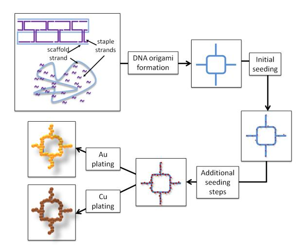
**Scheme 3.1** Fabrication and metallization of DNA origami. The process starts with the formation of DNA origami, which is deposited on a Si surface. Next, Pd seeding steps are done, during which Pd seeds grow on the DNA template. Then, either Au or Cu electroless plating is used to enhance and develop seeds into thicker and continuous nanostructures.
