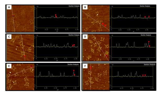
**Figure 3.3** Examples of AFM section analyses for samples of (A-F) 0-5 Pd seedings. In total, more than 100 measurements were done for each condition, which were used for height distribution analysis in Figure 3.2.
