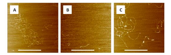
**Figure 2.3** The effect of  $Mg^{2+}$  on surface DNA attachment after DMAB reduction. AFM images of lambda DNA on mica (A) before DMAB treatment, (B) after DMAB treatment for 1 min with no added  $Mg^{2+}$ , and (C) after DMAB treatment with 5 mM  $Mg^{2+}$  in the reducing solution. Scale bars: 1  $\mu$ m; height scale: 5 nm.
