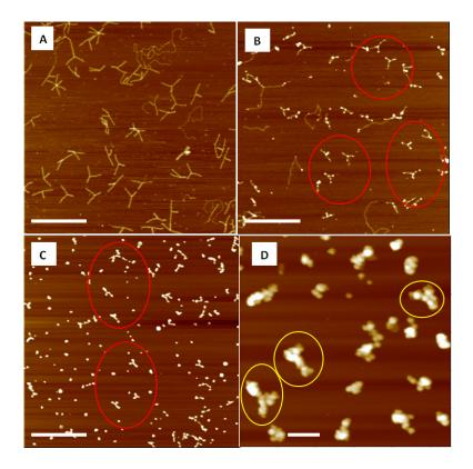
**Figure 2.6** AFM images of metallization of T-shape DNA origami on mica. (A) DNA origami. (B) Single Pd seeding. (C) Double Pd seeding. (D) Gold metallized. Scale bars for (A–C): 1  $\mu$ m. Scale bar for (D): 200 nm. Height scales for (A–C): 6 nm. Height scale for (D): 80 nm.
