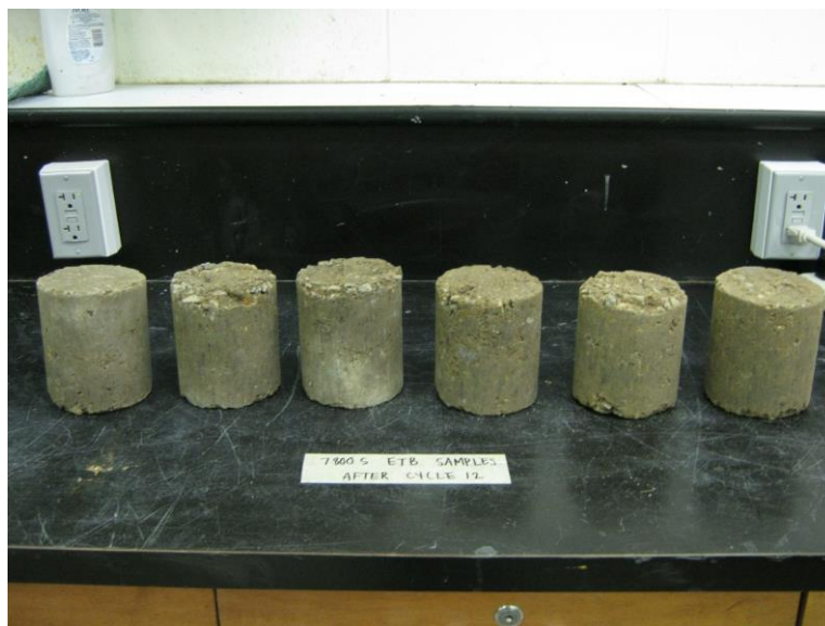
Figure 3-7: Freeze-thaw specimens from 7800 South.
