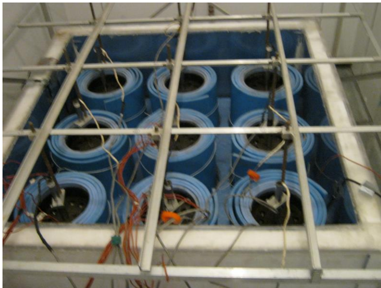
Figure 3-13: Frost heave test configuration.
