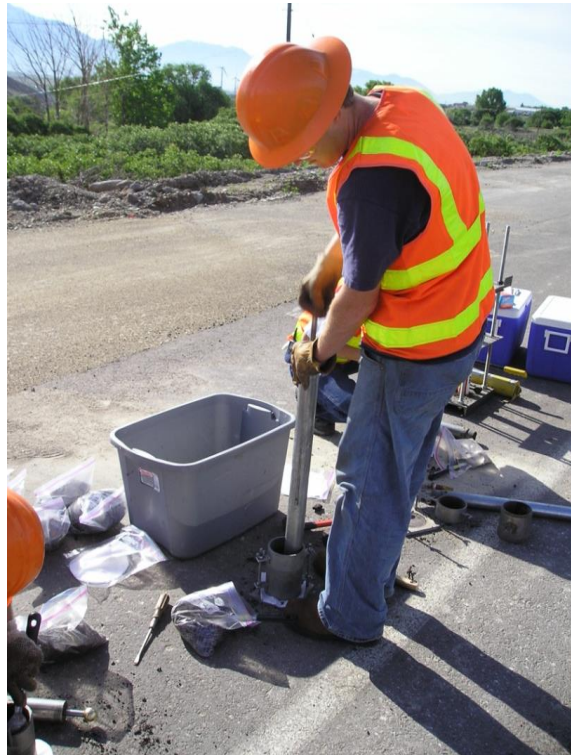
Figure 3-2: Compaction of emulsion-treated base specimen at Redwood Road.
