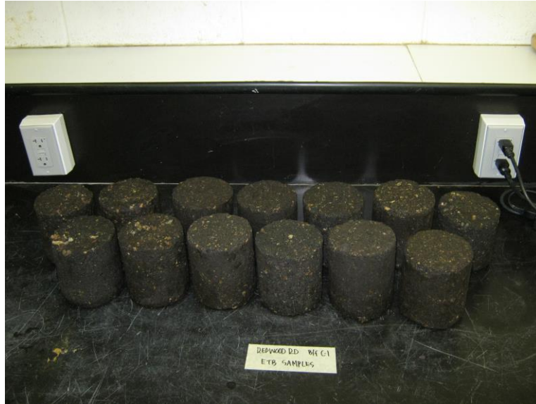
Figure 3-6: Freeze-thaw specimens from Redwood Road.
