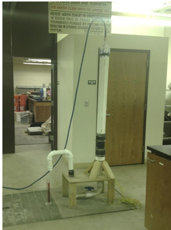
Figure 3-15. Permeability test configuration.
