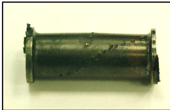
Figure 3-1: Gleeble Sample Localized Strain
