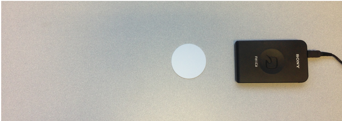
(a) Left: FeliCa NFC tag. Right: IC Card Reader/Writer and desktop computer.
