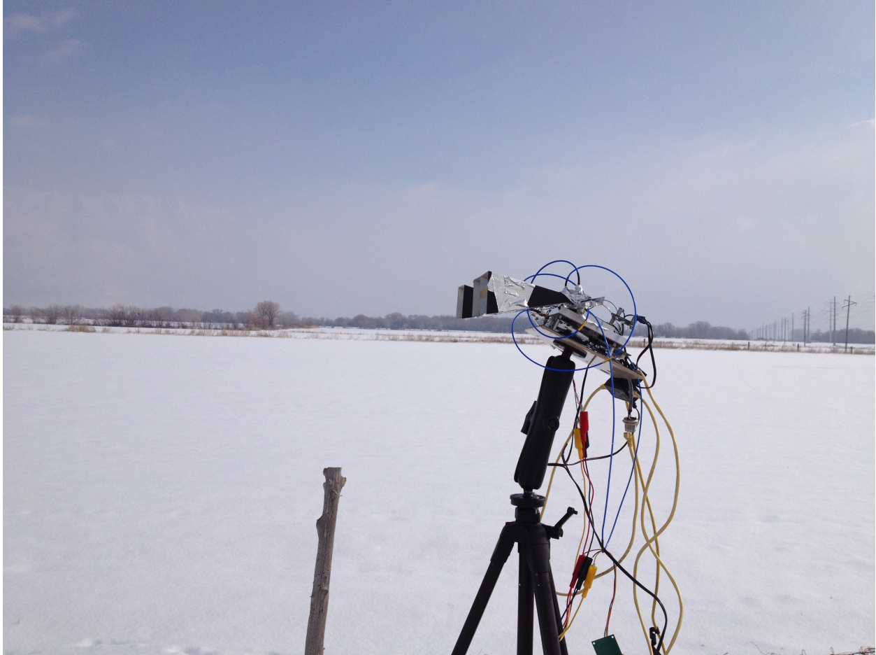
Figure 5.2: Data collection radar sitting on a tripod. Side view of the horn antennas and the cables.
