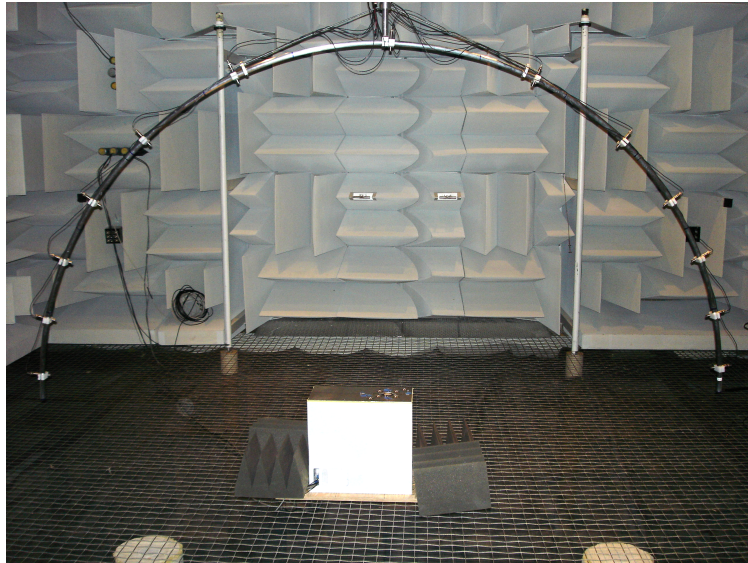
Figure 5.3 A boom microphone array used for far-field measurements.
