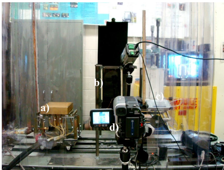
Figure 4.1. Flat-flame burner experimental set-up, including a) large flat-flame burner, b) cage with glass panel on each side, c) mass balance, d) video camera.
