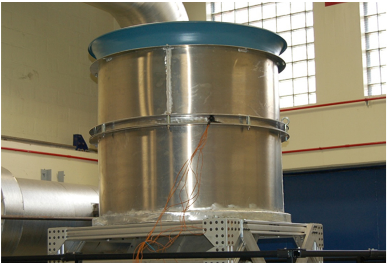
Figure 4.4: Flow barrel installation on model diffuser of ACF.
