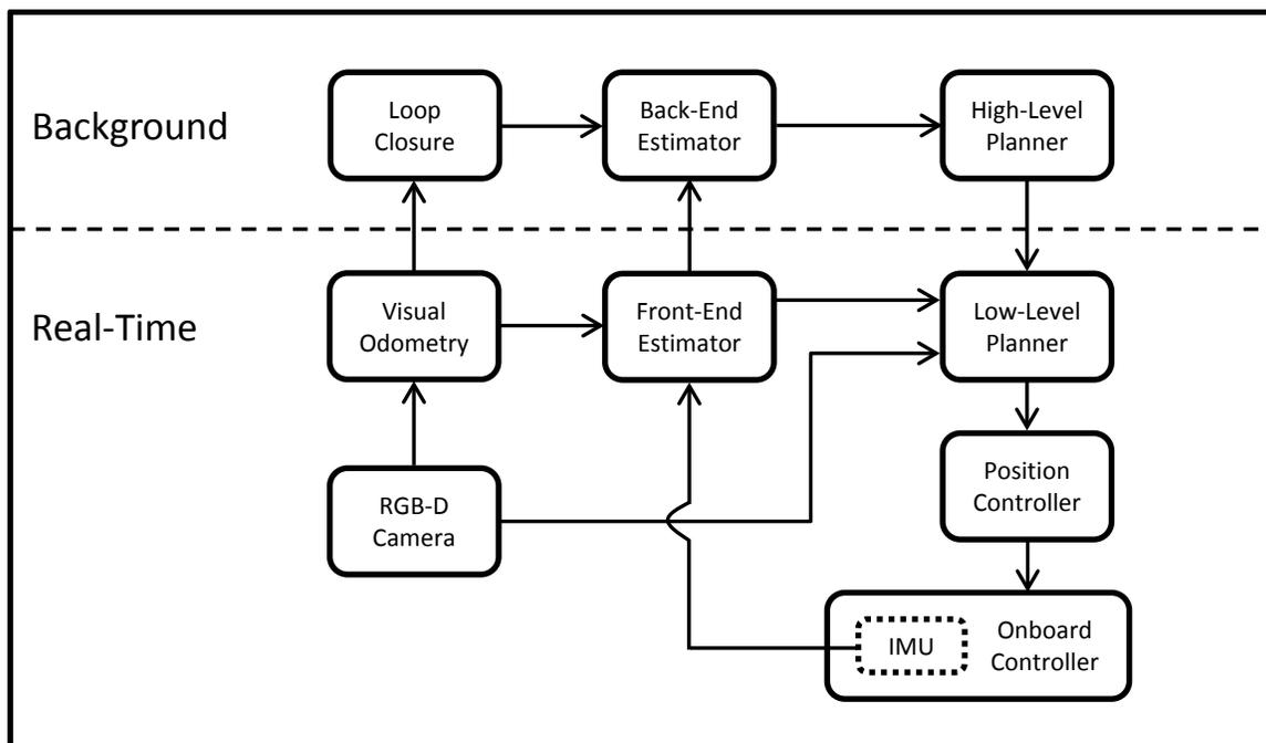
**Figure 1.7:** Our proposed navigation scheme. The system is based on graph-based SLAM. The time-critical navigation in the front-end is performed relative to reference frames associated with saved images of the environment. Refining the map happens when computational resources permit, and it only feeds directly into the vehicle’s high-level decision making.
