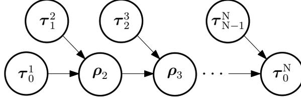
**Figure 3.3:** A Bayesian network based on the idea of using global poses as mediating variables, thus leading to the joint distribution  $p(\boldsymbol{\tau}, \boldsymbol{\rho})$ . Directed edges in the network are drawn to represent the physical reality that a relative transformation moves the vehicle from one global pose to another.
