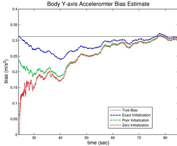
**Figure 2.8:** Estimates of  $\alpha_{j_b}$  over the first minute of flight. The true bias is marked by the solid black line at about  $0.31 \text{ m/s}^2$ . The three estimates plotted correspond to accurate (blue dashed), poor (green dash-dot), and zero (red dotted) initial calibration. After the estimates converge they remain close to the true bias for the duration of the flight.
