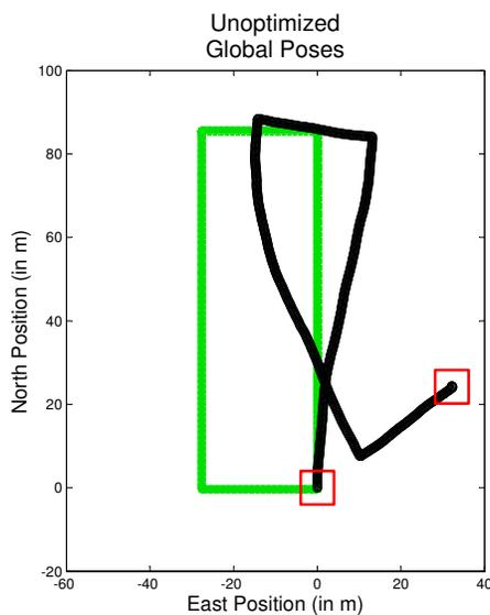
**Figure 3.4:** True global poses in green (gray) versus the unoptimized estimate (black) based on composed odometry-like transformations. Red boxed regions are shown close up in Figures 3.4 & 3.5.
