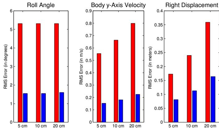
**Figure 2.7:** Average error in roll angles  $\phi$  and  $\phi_I$  (left), body y-axis velocity  $v$  (center), and relative right displacement  $r_L$  (right) over a four minute flight. Error of the traditional approach using (2.23) is graphed in red (light gray); error of estimates based on the improved model are graphed in blue (dark gray). Error is calculated for three scenarios differing in the level noise in the exteroceptive position update.
