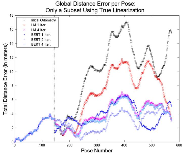
**Figure 4.12:** Global Pose Distance Error Using True Linearization Points in Algorithm 4. BERT achieves the most accurate solution at its second iteration.
