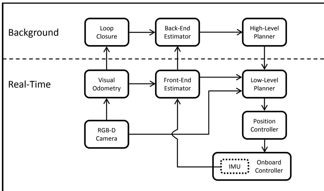
**Figure 5.1:** Our proposed navigation scheme. The system is based on graph-based SLAM. The time-critical navigation in the front-end is performed relative to reference frames associated with saved images of the environment. Refining the map happens when computational resources permit, and it only feeds directly into the vehicle’s high-level decision making.
