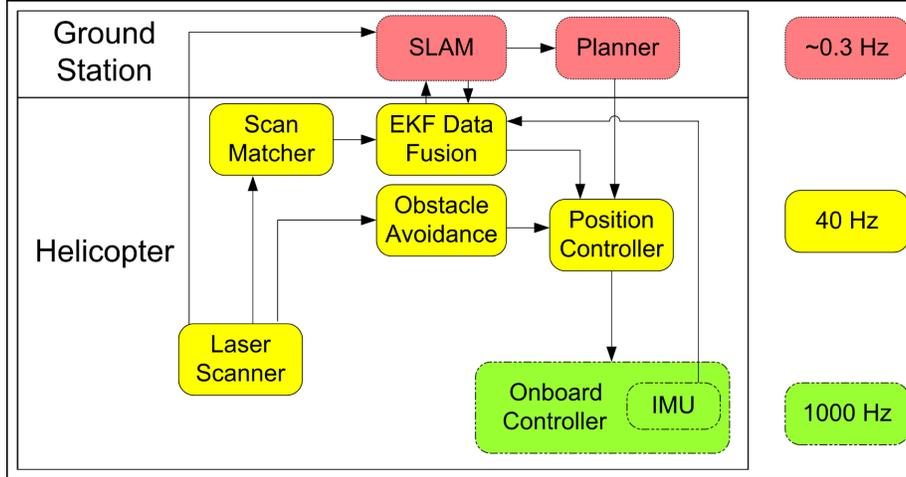
**Figure 1.5:** Estimation scheme used by [2] (© 2011 IEEE; used with permission). The important element to note is the simple distinction between processes required for real-time operation and those that are less critical.
