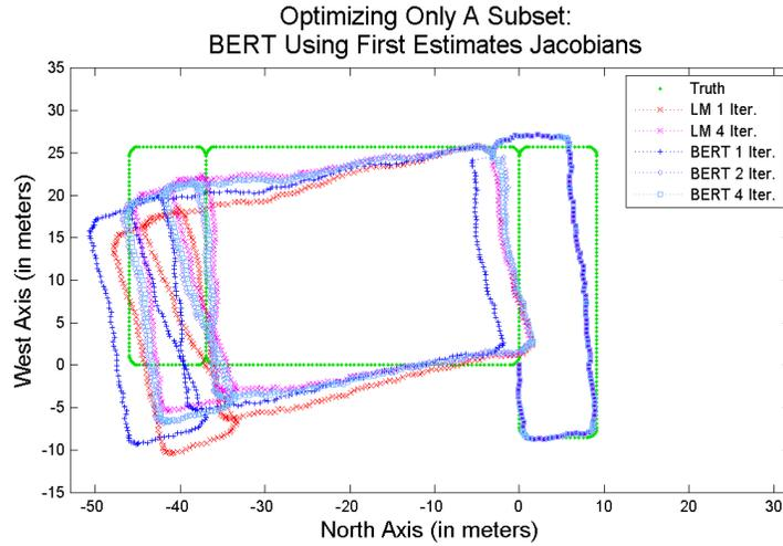
**Figure 4.15:** Overhead View of Optimized Poses Using FEJ Linearization Points in Algorithm 4. Notice that despite using unoptimized values to compute Jacobians BERT arrives at a solution essentially the same as LM. This suggests that an observability analysis similar to that of [45] might reveal even better linearization points and better results. However, an FEJ approach provides a reasonable result without any additional computation.
