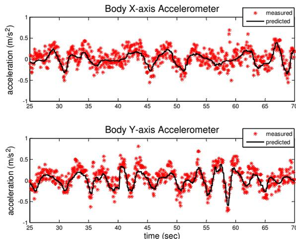
**Figure 2.2:** Actual accelerometer measurements for a nominal indoor flight plotted against those predicted by (2.9) and (2.10).
