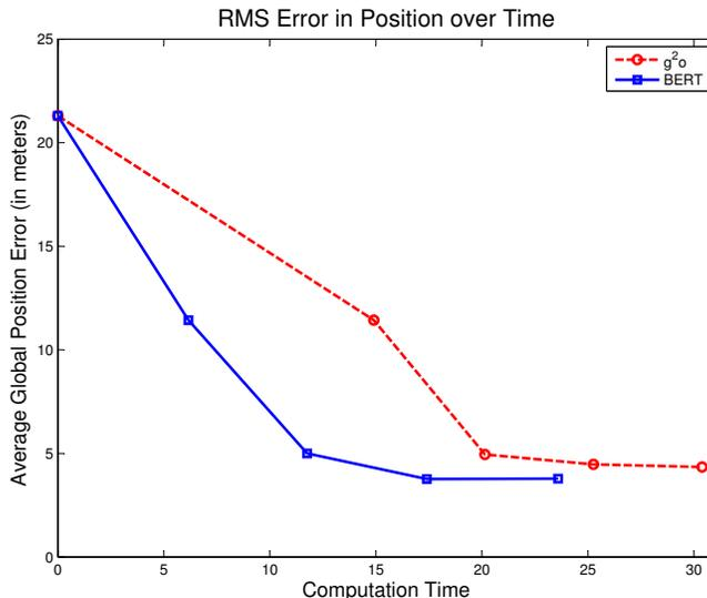
**Figure 3.13:** RMS Error in global position estimates as a function time accumulated over iterations of BERT and  $g^2o$ . Times shown for  $g^2o$  are given after subtracting all the linearization time out of each iteration; actual execution may be longer.
