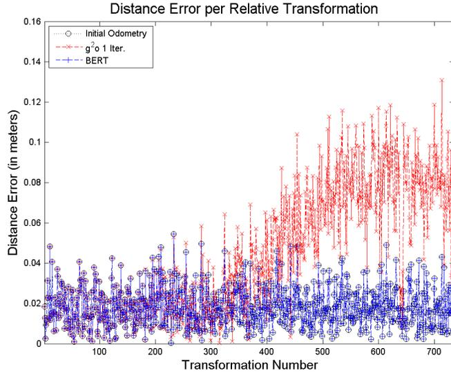
**Figure 3.8:** The error in distance for each relative transformation estimate. We should expect optimized estimates to change only slightly from the originals because the 735 independent odometry-like transformations are being updated with information from a single loop closure. The important feature to note is the degradation toward the end of the trajectory caused by one iteration of  $g^2o$ .
