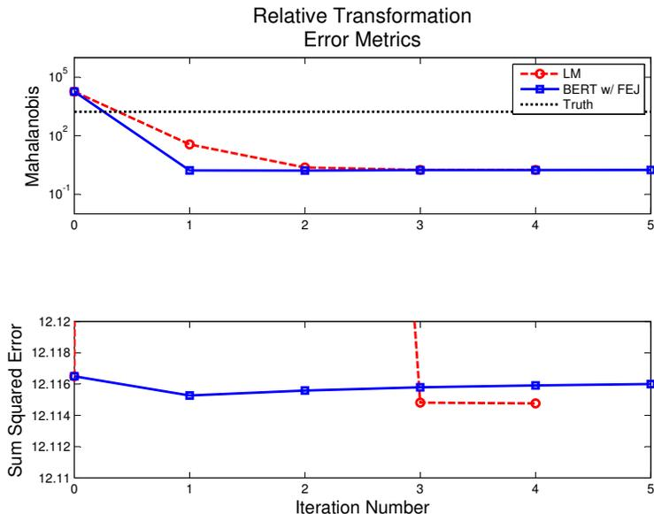
**Figure 4.17:** Relative Transformation Error Metrics Using FEJ Linearization Points in Algorithm 4. Performance is similar to that shown in Figure 4.12 where true state values were used in linearization.
