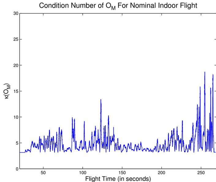
**Figure 2.3:** This figure shows the condition number of the observability matrix as a function of time for a nominal indoor flight. The condition number is defined as the ratio of the largest to the smallest singular value of  $\mathbf{O}_M$ . This figure represents the condition number for  $\mathbf{O}_M$  without approximations other than neglecting terms multiplied by gyroscope biases.
