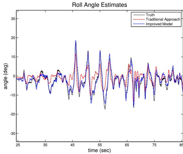
**Figure 2.4:** Estimates of roll angle,  $\phi$ , during the first minute of a manually controlled flight. This results were generated using exteroceptive position updates arriving at 5 Hz, delayed on average by 250 ms, and with 5 cm standard deviation of error. Flight begins at about  $t = 25$  seconds.
