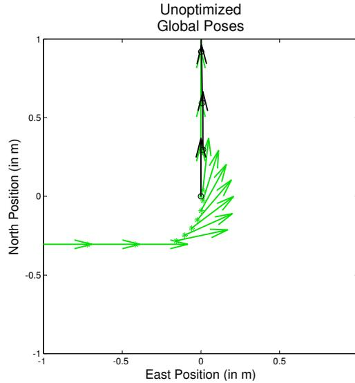
**Figure 3.5:** A close up view of Figure 3.3 around the true beginning and end of the trajectory, where loop closure occurs. Arrows indicate the true (green/gray) and estimated (black) heading; the corresponding positions are marked (green/gray stars; black circles) at the base of each arrow.
