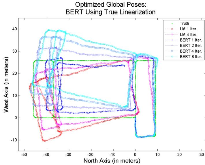
**Figure 4.8:** Overhead View of Optimized Poses Using True Linearization Points in Algorithm 3. Compared to the results in Figure 4.5, BERT now converges to a solution resembling truth, though less accurate than the LM solution.
