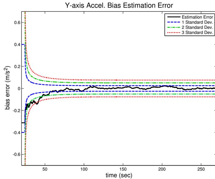
**Figure 2.9:** Error of the  $\alpha_{j_b}$  estimate over the entire flight when initialized to zero (i.e. uncalibrated). The error is plotted as the solid black line. The remaining curves designate multiples of the marginal standard deviation of the error as calculated by the filter.
