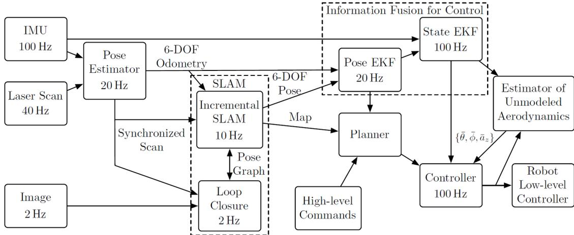
**Figure 1.4:** Estimation scheme used by [1] (© 2011 IEEE, used with permission). While the scheme is demonstrably effective, it is a little confusing to follow. We believe a more simple scheme can be developed based on principles described below and in Section 1.2.
