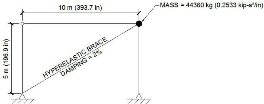
**Figure 3-1: Frame model used in SDOF analysis.**
