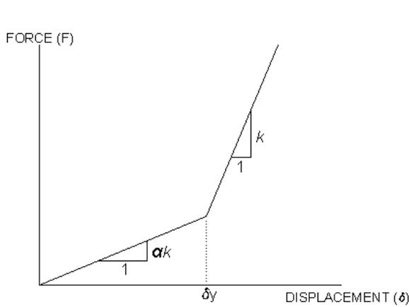
**Figure 3-2: Parameters used to describe behavior of stiffening elastic system.**
