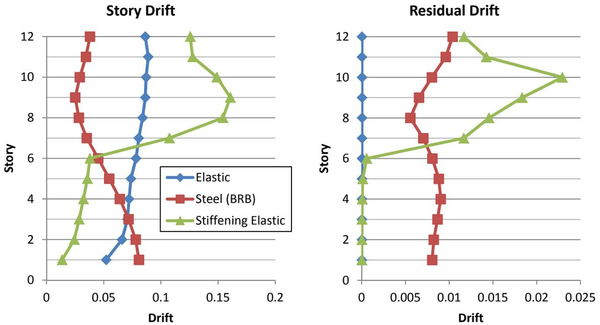
Figure 4-5: Story drift and residual drift of the model with stiffening elastic systems on the lower half.
