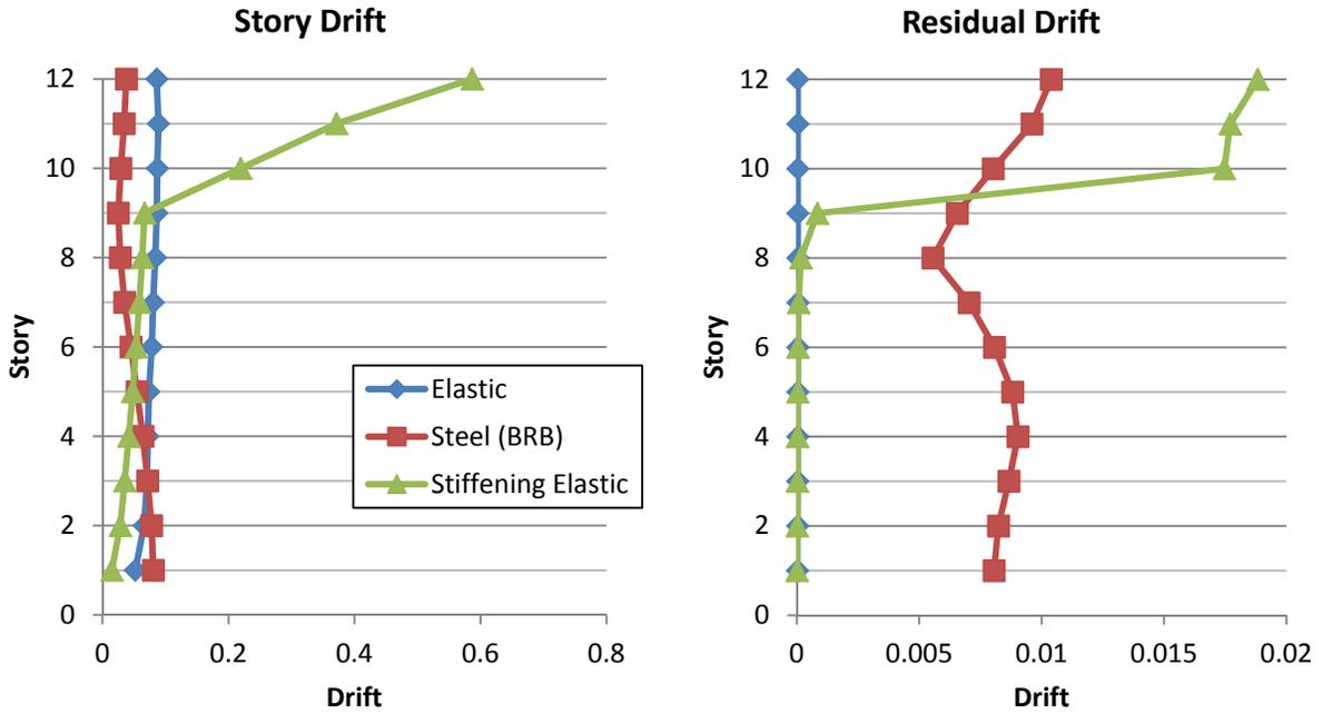
Figure 4-6: Story drift and residual drift of the model with stiffening elastic systems on the lower nine floors.
