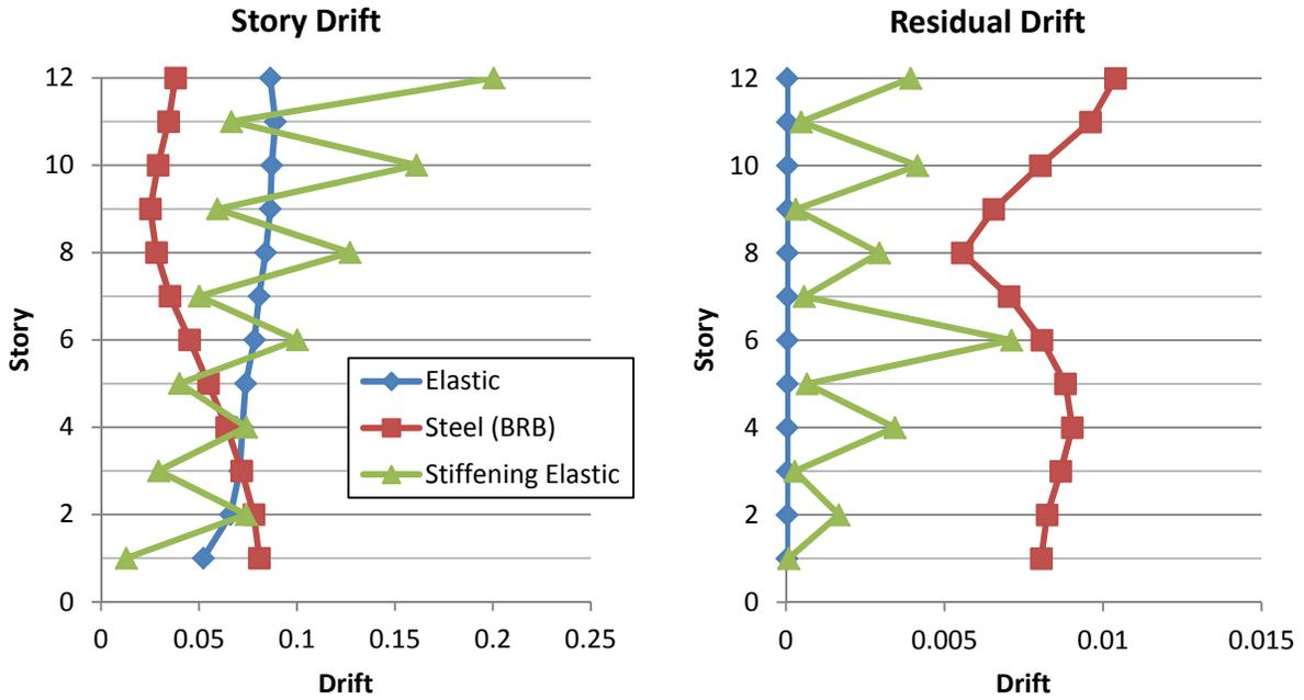
Figure 4-4: Story drift and residual drift of the model with alternating stiffening elastic and BRBF systems.
