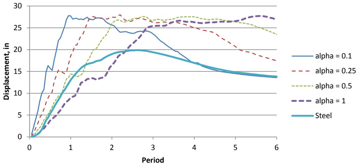
Figure 3-10: Average displacement spectra for  $\delta_y = 25$ .
