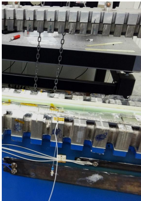
Figure 5-6: A completed sensor setup that is ready for the upper containment half to be placed atop.
