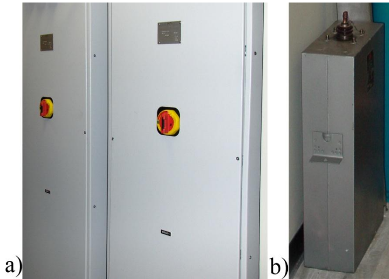
Figure 5-4: Two of the three capacitor banks (a) that power the railgun and single capacitor (b).
