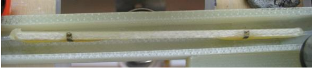
Figure 4-11: A suspension mounted SCOS in an FR4 cartridge.
