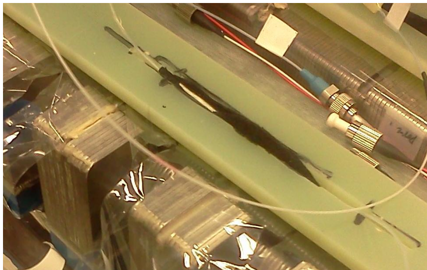
Figure 5-11: A SCOS sensor placed inside of an insulator using foam.
