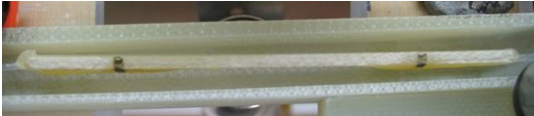
Figure 5-17: A SCOS inside of a three sided cartridge.
