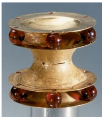
Figure 2-7: The original ion trap developed by Wolfgang Paul. Figure from http://bigs.physics-astro.uni-bonn.de/index.php?id=76
