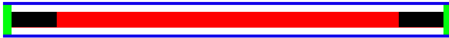
Figure A-1: Stencil for the laser cutter at the BYU Electrical Engineering shop. The width is 5 cm and the height is 0.4 cm.
