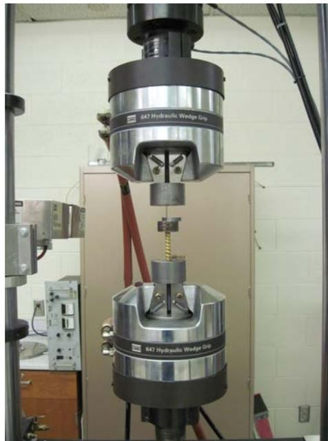
**Figure 2.9: Instron Test Machine**
