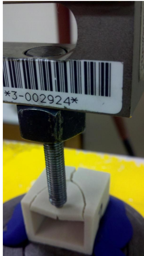
Figure 5.1.3 Z Corp. Cubic Specimen Being Tested to Failure
