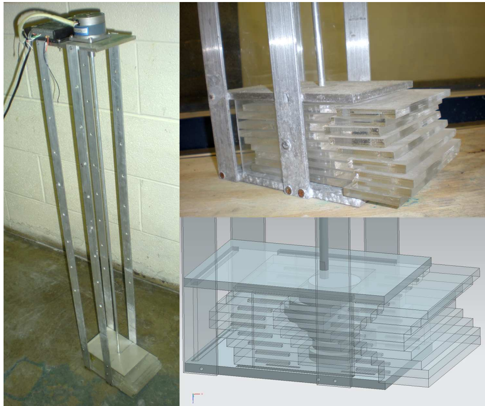
Figure 3.3: Left: The completed wave generator. The nine acrylic plates are at the bottom of the generator and 4 supports extend up to the top motor mount plate. A shaft extends from the motor to the cams within the plates. Top Right: Close up image of the nine plates creating a sinusoidal profile. Bottom Right: Transparent depiction of a wave generator allowing the cams inside the plates to be seen.
