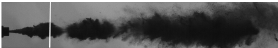
Figure 2.8: Representative image of how the intensity of a single column of pixels (white line) at a fixed distance downstream from the nozzle is used to measure the frequency of pulsation.
