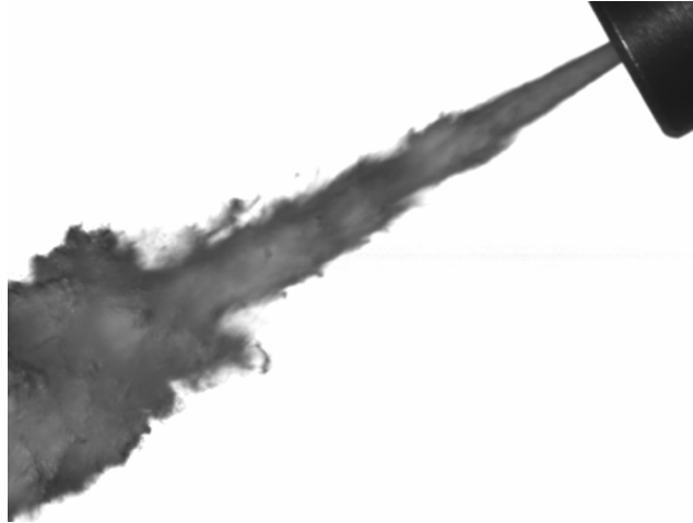
(a) Cavitating water jet: 1.0 mm nozzle, 20.7 MPa
