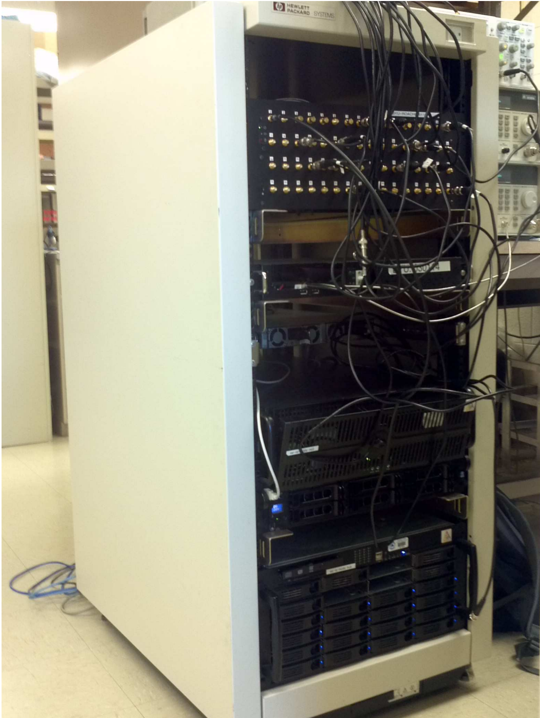
Figure 5.4: A view of the instrument rack with ROACH boards, a host computer and a server computer.
