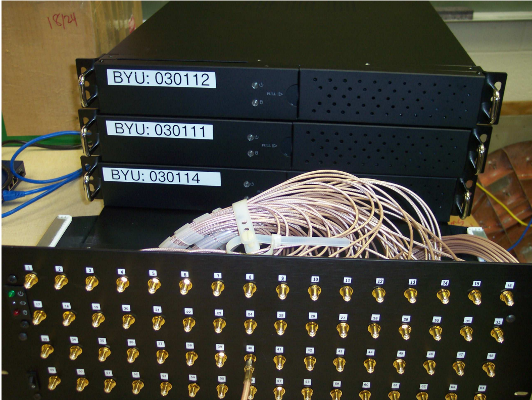
Figure 5.3: Image showing the front view of all the ROACH boards. The bottom ROACH board shows the front panel of the board having the inputs for the x64 ADC.
