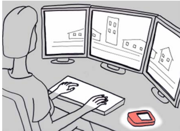
Figure 1:13 – Desktop interaction. All application processing happens within the handheld (to the right of the user).
