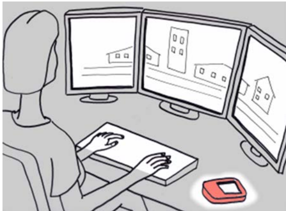
Figure 2:3 – Desktop interaction. All application processing happens within the handheld (to the right of the user).
