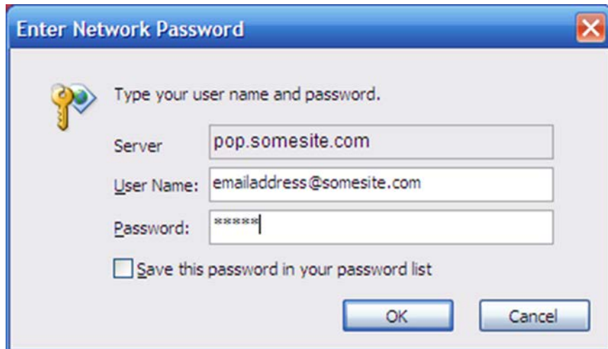
Figure 3:2 – An inappropriate dialog for a public display—it shows private information. The display now has the user’s email server, email address, and password length.
