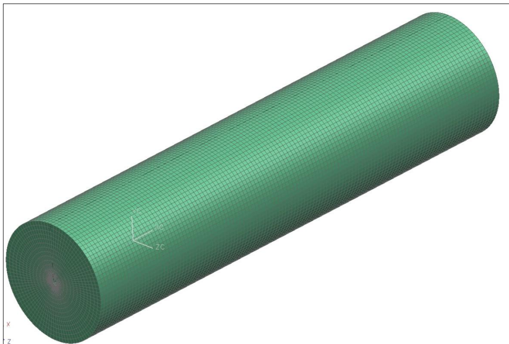
Figure 4-20: 3D Hexagonal Mesh of Simple Example
