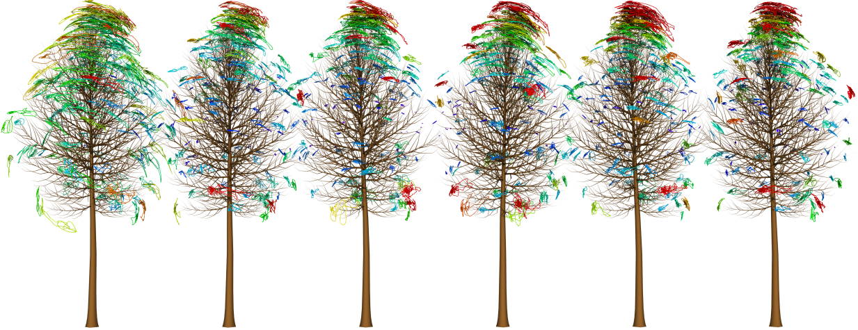
Figure 4.2: 1200 branch motion paths on 6 trees (200 per tree) after a 12-15 m/s wind event using a 1.6m grid for fluid simulation and a turbulence model based on strain estimation and the Kolmogorov cascade.
