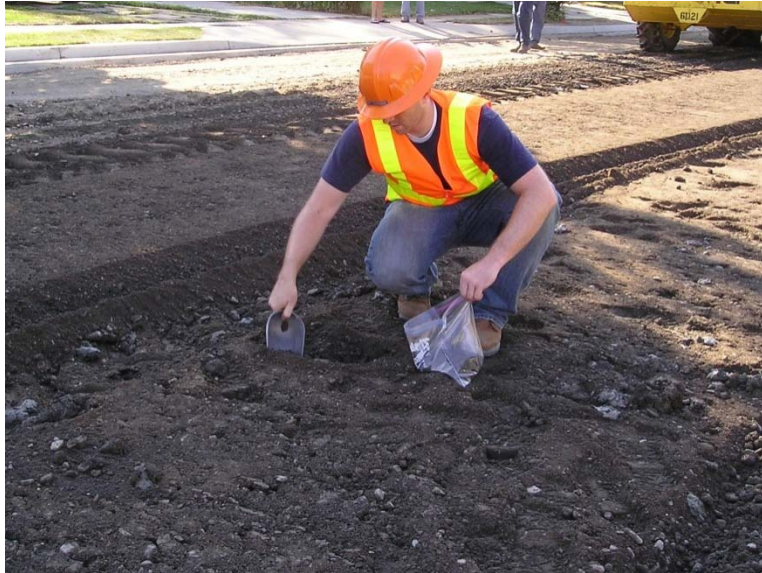
Figure 3-7: Sampling of RAP-base blend.
