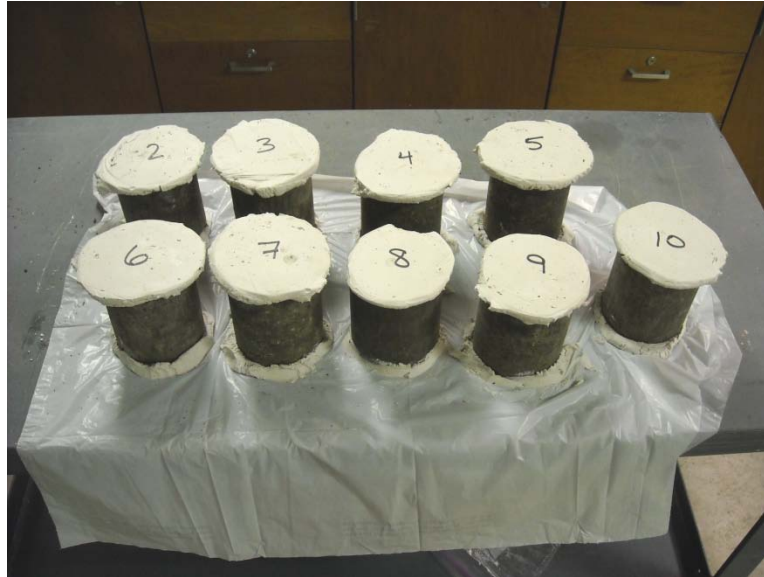
Figure 3-12: Capping field specimens.
