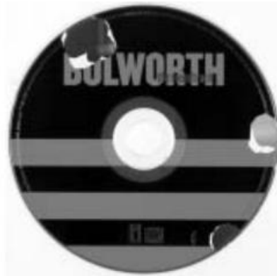
Figure 2-15: Audio CD Delaminating after 84 Days of Aging (Iraci 2005)
