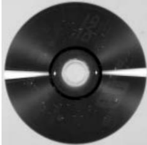
Figure 2-11: Example of Pinholes in Reflective Layer (Iraci 2005)
