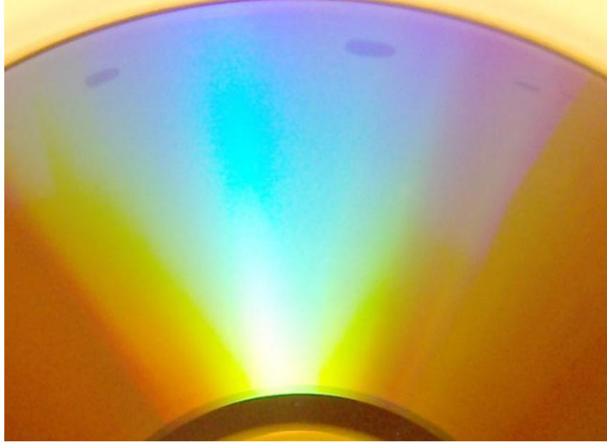
Figure 4-11: MI1 Black Spot Defects at 24 Hours
