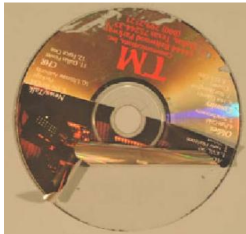
Figure 2-14: Metal Layer Separating From Substrate (Shahani, Manns and Youket 2004)
