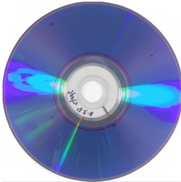
Figure 4-6: Four Mark Disc Image Overlaid on POF Errors
