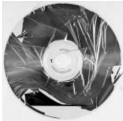
Figure 2-16: CD-R Delamination after 21 Days of Aging (Iraci 2005)
