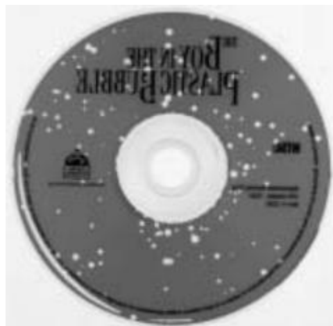
Figure 2-10: Example of Pinholes in Reflective Layer (Iraci 2005)
