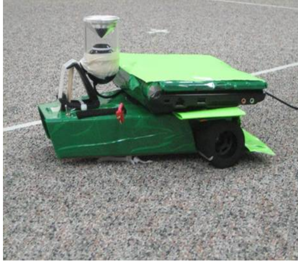
Figure 2.15: The Stinger robot. This robot is equipped with a controller, two wheel encoders, an omnidirectional camera, and Asus EEE computer.
