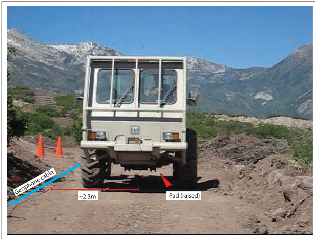
Figure 9 - Photo facing east on seismic line 9. The vibroseis vehicle (IVI Minivibe) with approximately 6 ft (~2.3 m) offset from the geophones. (Photo by Bill Keach, 2007)
