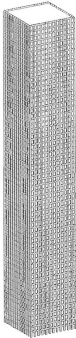
Figure 1-4: Exterior Frame Tube in Tube
