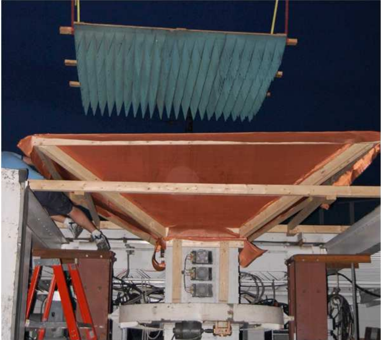
Figure 4.8: Absorber being lowered into the ground screen
