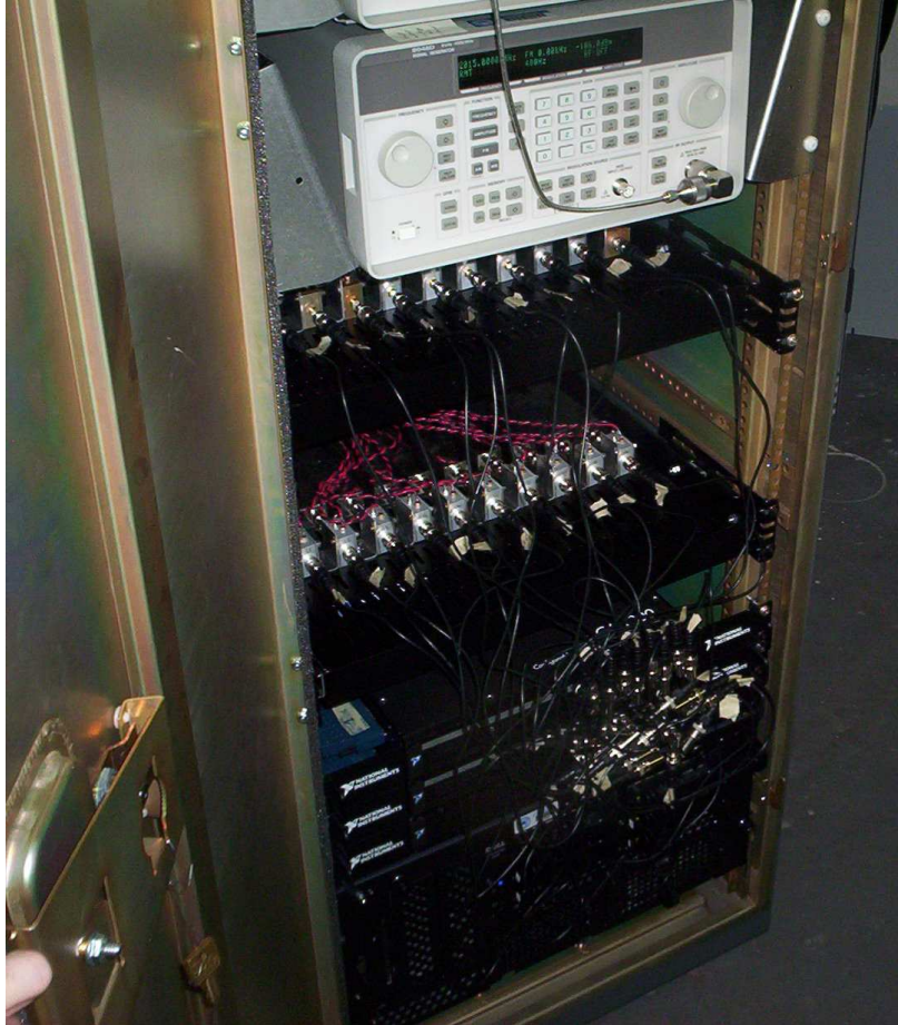
Figure 3.8: Shielded rack holding the digital back end and signal generators for LO signals. A single server-class PC holds 5 ADC cards with 4 inputs per card for a total of 20 synchronously sampled inputs at 1.25 Msamp/sec. All data are streamed to disk for post-processing.
