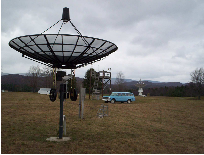
Figure 3.9: 3.6m reference antenna in front of RFI enclosure for positioner control boxes, with the Green Bank 20 Meter Telescope in the background.
