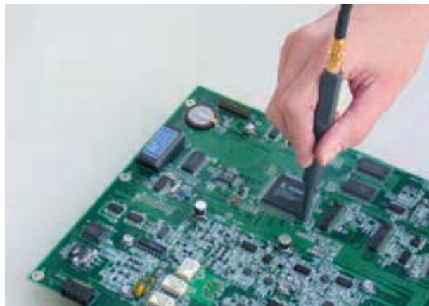
Figure 1-1: B&K PR 26M magnetic field probe.
