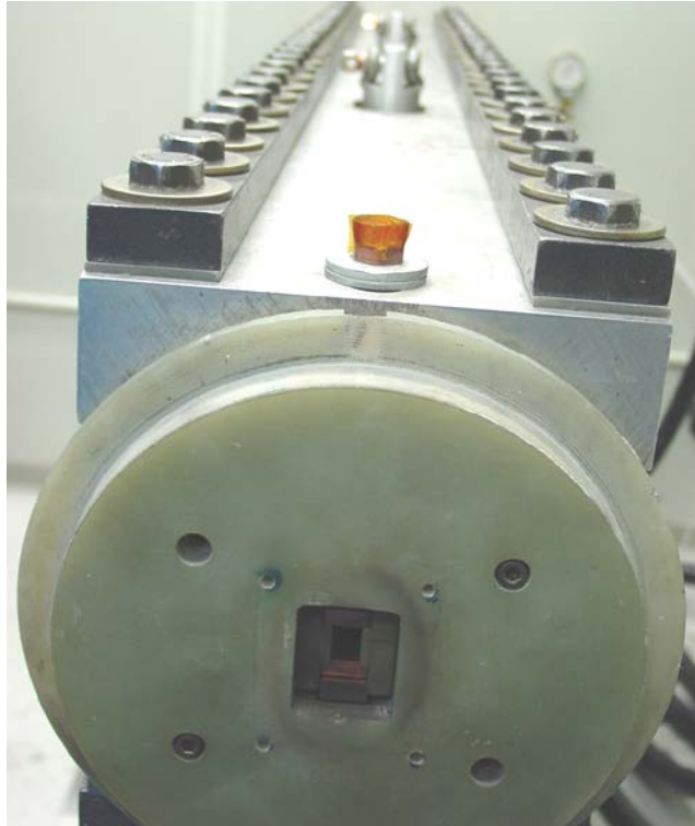
Figure 5-4: The large rail gun enclosure system used to limit vibrations. The small hole in the center is where the projectile launches and the copper rails can be seen above and below the hole.
