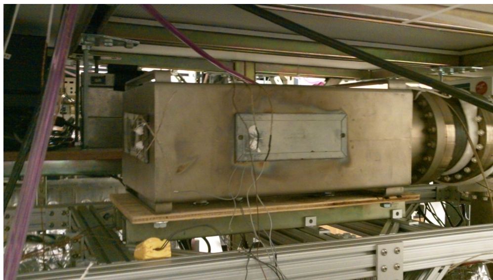
Figure E.3 Picture showing the location of the plate heaters on the ion pump. The magnet was removed from the pump in order to reach temperatures above its Curie temperature.
