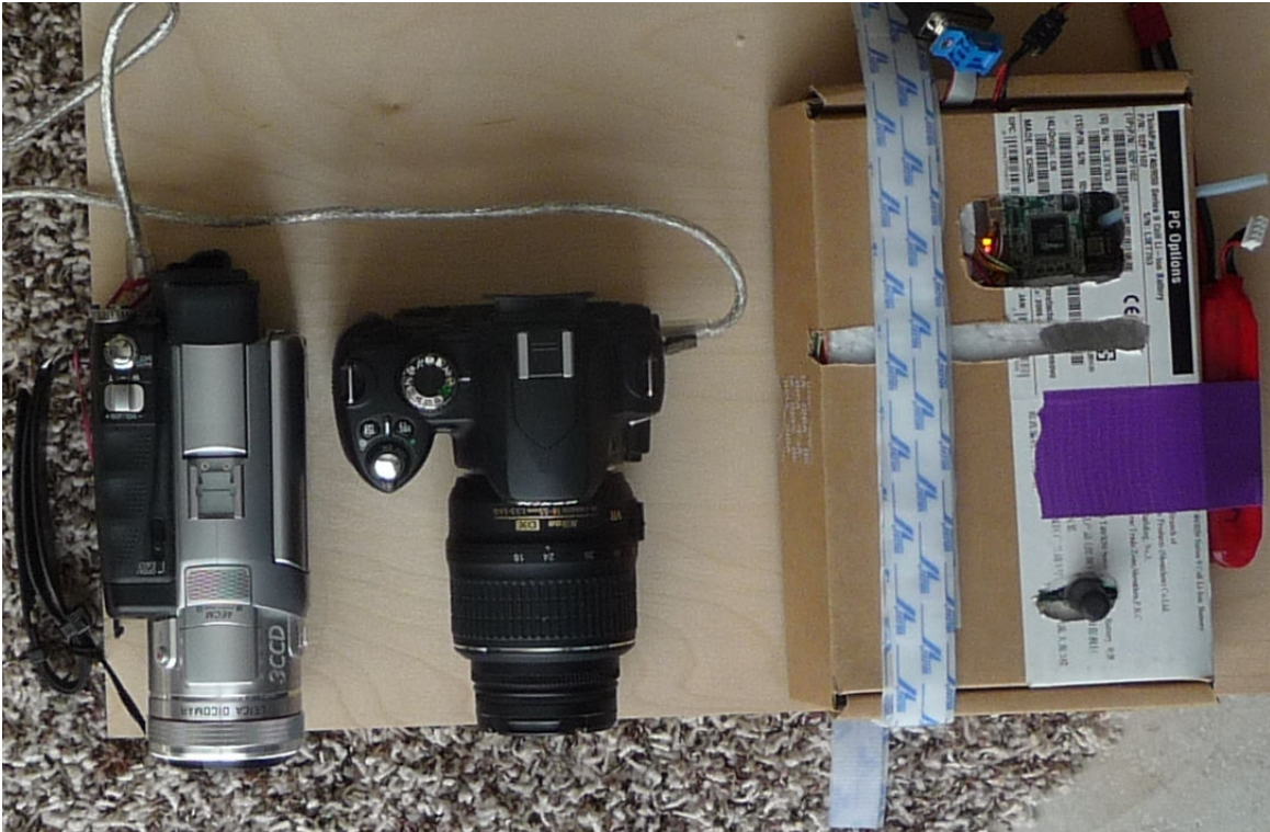
Figure 3.4: Camera Rig Prototype. The primary camera, secondary camera, and telemetry units are shown from left to right.
