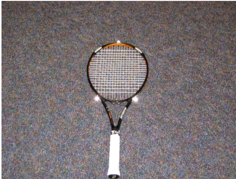
Tennis racket with markers on each shoulder and one on the tip
