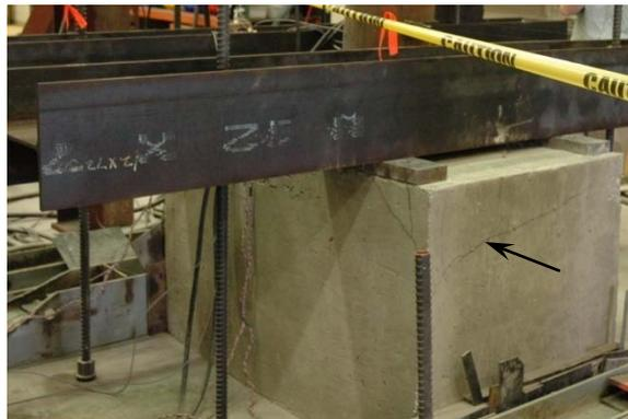
**Figure 4-11: Cracking at the End of Specimen 3 (North-South)**
