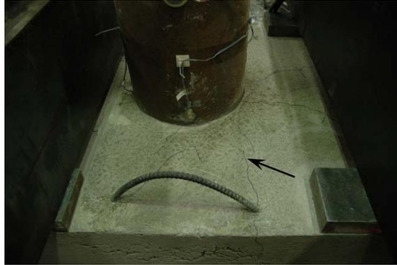
**Figure 4-12: Specimen 3 After Testing (East-West)**
