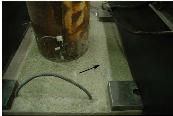
**Figure 4-6: Initial Cracking of Specimen 2 (East-West)**
