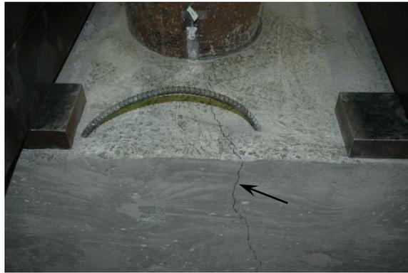
**Figure 4-2: Initial Cracking in Specimen 1 (East-West)**
