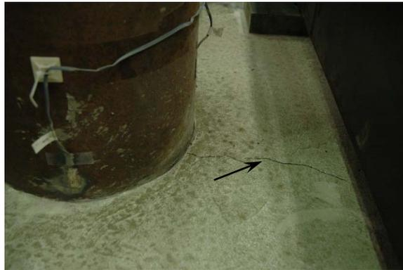
**Figure 4-10: Initial Cracking of Specimen 3 (East-West)**
