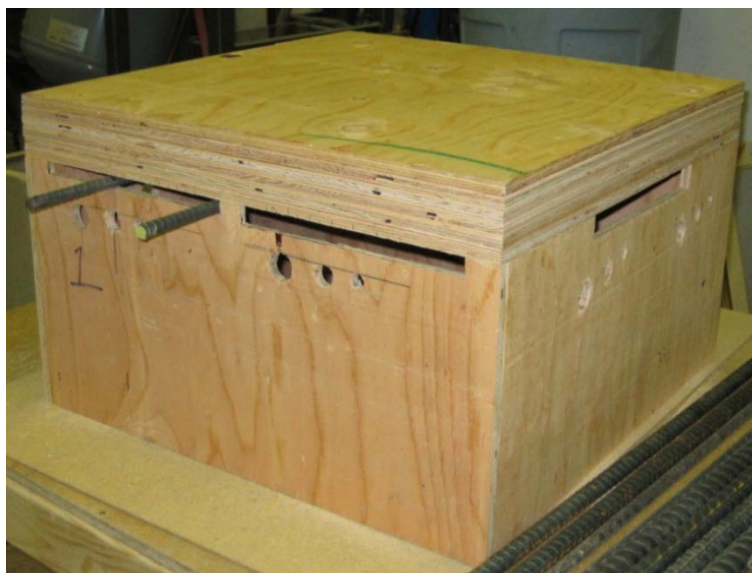
Figure 3-3: Rebar configuration for FOV experiment.
