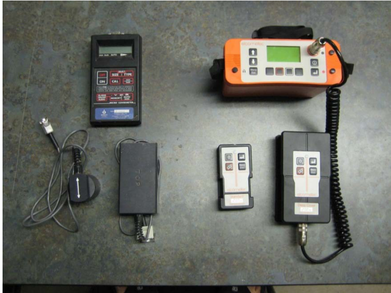
Figure 3-1: Cover meter 1 and 2 with deep and shallow antennas.
