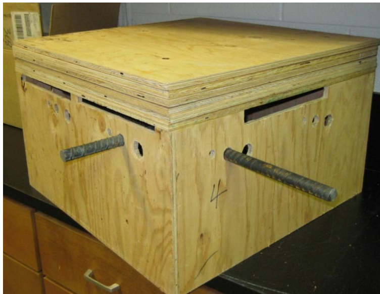
Figure 3-4: Rebar configuration for PTAI experiment.
