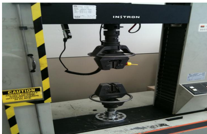
Figure 3-5 Instron Tension Machine Used for Mechanical Testing
