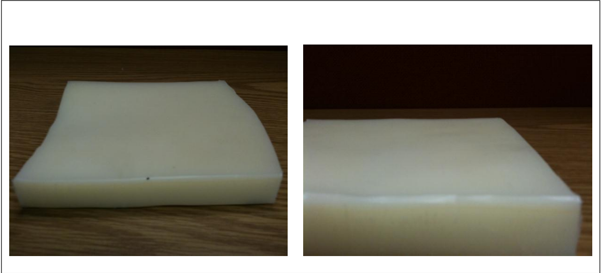
Figure 4-2 Interior Surfaces of Virgin Samples Showing no Surface Defects
