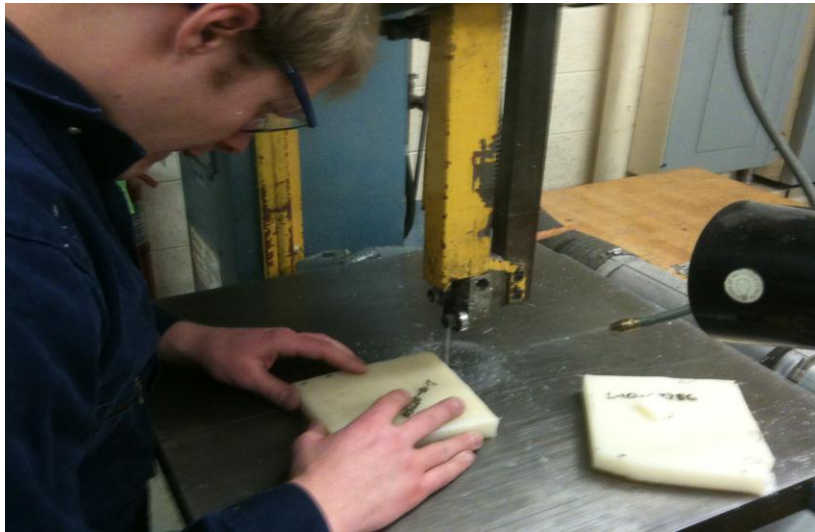
Figure 3-3 Bandsaw Cutting Samples
