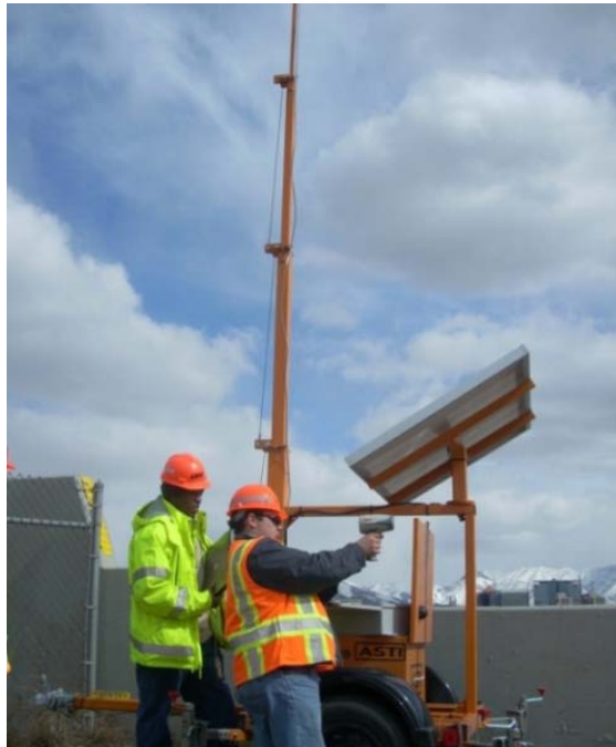
Figure 3-4 Sensor calibration using radar gun (taken by Mitsuru Saito).
