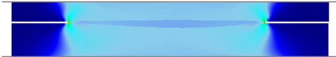
Figure 59: Postprocessed Final Simulation Time Step (Effective Stress Plot)
