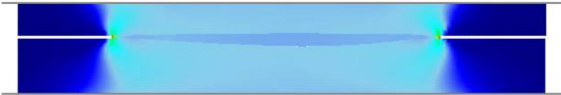
Figure 75: DEFORM Postprocessed Final Simulation Time Step (Effective Stress Plot)
