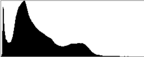
Figure 4.8: Histogram of original image. Pixel brightness is skewed and not evenly spread across spectrum.
