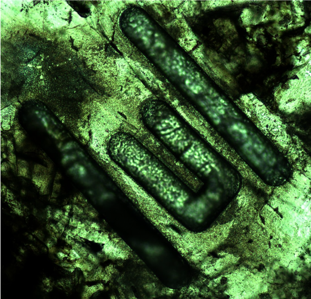
Figure 17. Image of grain HI-205 Plagioclase 3 following LA-ICPMS. In this image there is a "U" shaped trough in the center of the grain where the core was ablated and two parallel troughs on either side of the grain where rim samples were taken.
