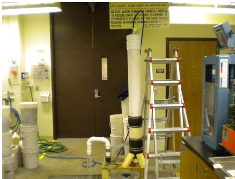
Figure 3.8: Typical hydraulic conductivity test configuration.
