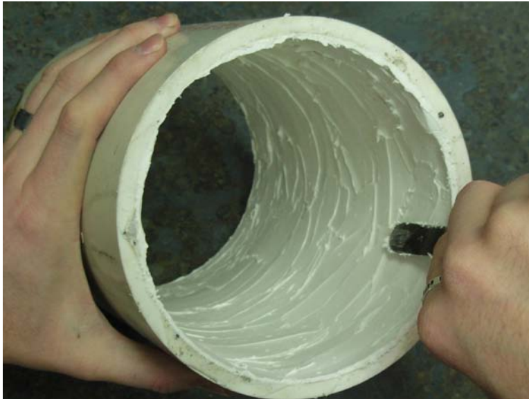
Figure 3.6: Sample mold for hydraulic conductivity testing.
