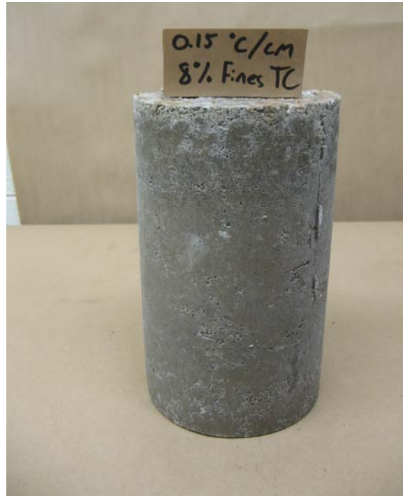
Figure A.14: Specimen with 8 percent fines tested with thermocouples at thermal gradient of 0.15^{\circ}\text{C}/\text{cm} .
