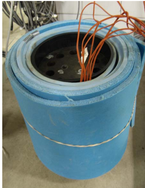
Figure 3.3: Sample with insulation and overburden weight.
