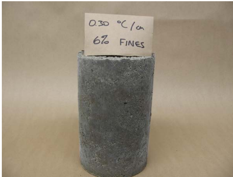
Figure A.18: Specimen with 6 percent fines tested with thermocouples at thermal gradient of 0.30^{\circ}\text{C}/\text{cm}
