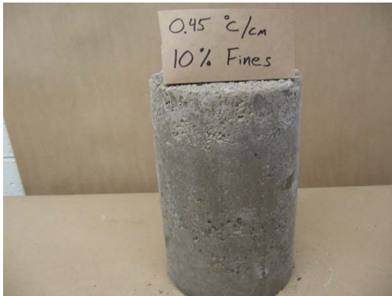
Figure A.27: Specimen with 10 percent fines tested without thermocouples at thermal gradient of 0.45°C/cm.
