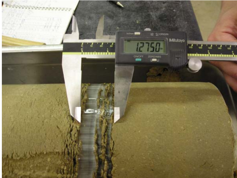
Figure 2.2: Ice lenses in a Montana silt (35).
