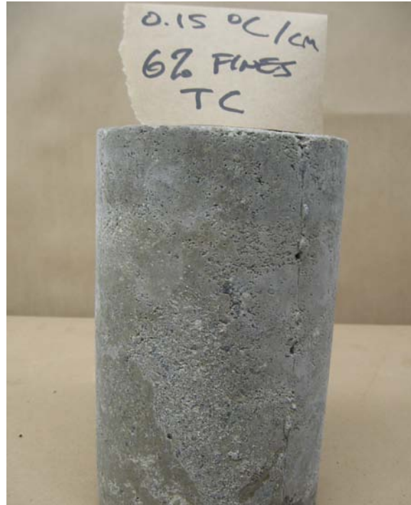
Figure A.12: Specimen with 6 percent fines tested with thermocouples at thermal gradient of 0.15^{\circ}\text{C}/\text{cm} .
