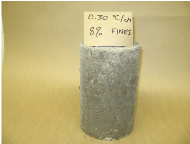
Figure A.20: Specimen with 8 percent fines tested with thermocouples at thermal gradient of 0.30^{\circ}\text{C}/\text{cm} .
