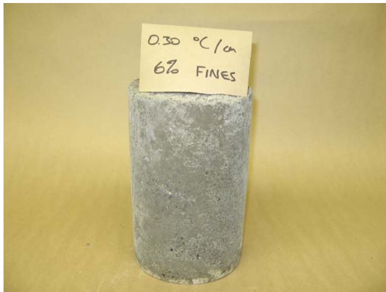
Figure A.17: Specimen with 6 percent fines tested without thermocouples at thermal gradient of 0.30^{\circ}\text{C}/\text{cm}
