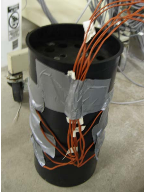
Figure 3.2: Sample instrumented with thermocouples.
