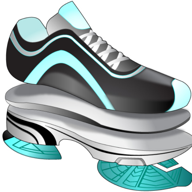
Figure 2.2: A shoe, with an exploded view of the layers of the shoe sole
