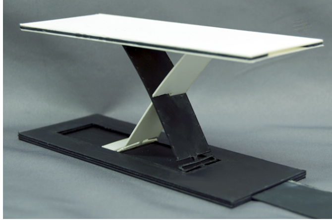
Figure 3.17: MLEM Nuremberg scissor mechanism used to separate layer
