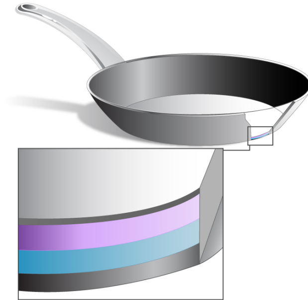
Figure 2.3: A frying pan, with a section cut away and a zoomed-in view of the base layers of the frying pan
