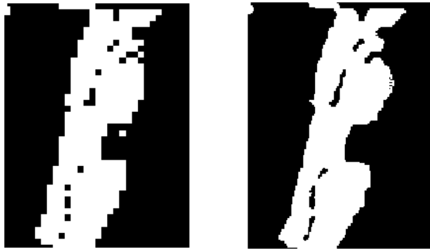
Figure 5-5 : Initial defect map (left) and after scan refinement (right).
